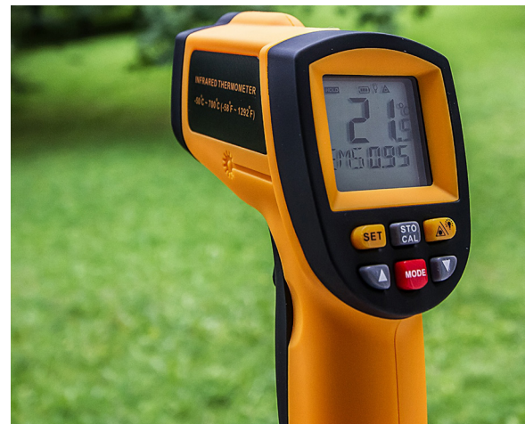
Figure 5: This digital thermometer automates the process of digital reading traditionally carried out by a human peering at the gradations marked along the side of a tube containing mercury or alcohol. Image created by Wikimedia user Hedwig Storch, used under license CC BY-SA 3.0 ( https://creativecommons.org/licenses/by-sa/3.0/ ).
