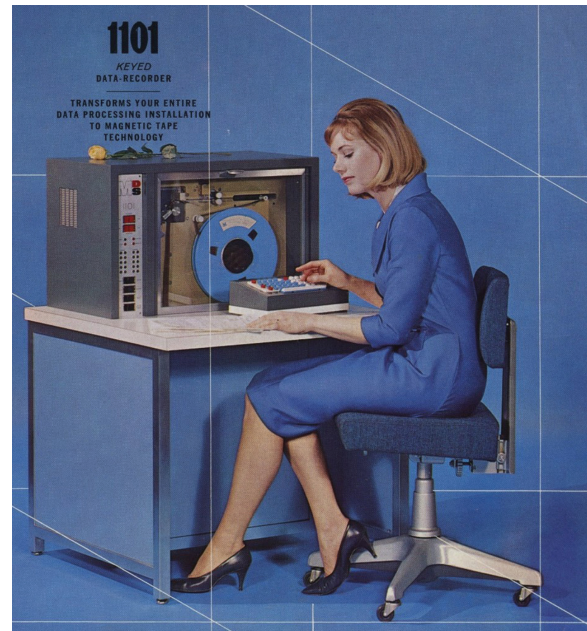
Figure 2: A key to tape unit, introduced by Mohawk Data Systems in 1965. 2
